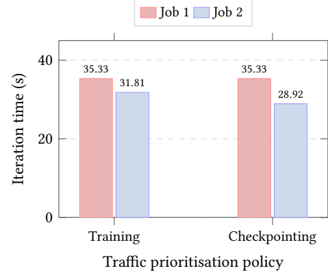
Figure 7: Prioritising checkpointing traffic reduces Job 2 iteration time without affecting Job 1, since checkpointing is prioritised over non-critical data-parallel communication.
