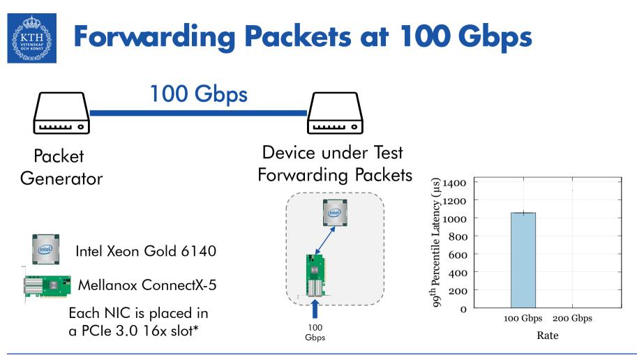
\* A PCIe 3.0 16x slot is capable of providing ~125 Gbps effective full-duplex bandwidth.
